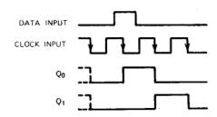
Note 6: Output switching characteristics may not satisfy the ratings if the clock signal is applied without observing the set-up time.
